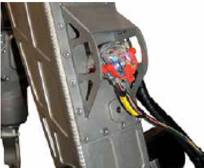
In-arm electronics are located in the forearm, increasing system reliability and minimizing electrical connections
